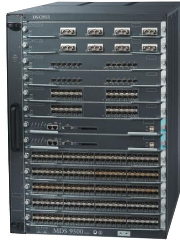
The Cisco MDS 9513 for IBM System Storage offers 1, 2, 4, 8 and 10 Gbps link speeds with up to 528 Fibre Channel ports in a 14U enclosure
