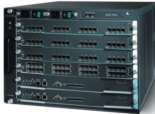
The Cisco MDS 9506 for IBM System Storage offers 1, 2, 4, 8 and 10 Gbps link speeds with up to 192 Fibre Channel ports in a 7U enclosure
