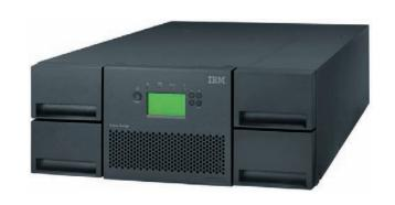
The TS3200, featuring full- and half-height technology offers 8 Gbps Fibre Channel for LTO Ultrium 7, 6, 5, and 4 and 6 Gbps SAS interfaces for LTO Ultrium 7, 6, 5 and 4. It can be attached to a wide variety of open-system servers. The sequential or random-access library comes in a standalone or optional rack-mountable configuration. The TS3200 also has an LCD display and indicators for power, drive and activity, error status and message information.
